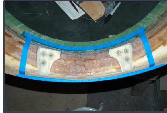
Pot In Threaded Inserts & Tape Off Tacky Tape Locations
